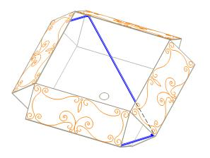
The cardboard box is hinged to allow it to pop—up. The action is cause by elastic bands that runs to opposite corners (only one is shown for clarity). In each corner is sewn some plastic rings that cause the corners to keep proper alignment.
